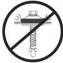
INCORRECT Excess overtightening
